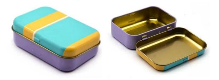
2. Technical Specifications Dimensions: 98mm (L)  $\times$  68mm (W)  $\times$  29mm (H) Material: 0.23mm thick tinplate with food-grade lacquer coating . Hinged Lid: Reinforced steel wire hinge for 10,000+ open/close cycles . Surface Finish: Matte or gloss varnish, UV printing, and anti-scratch coatings .
